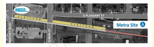
Illustrates a 10-car consist fitting all doors on an 805-ft. split platform. Doors are mid-car, so engineers stop with doors on platform as illustrated here.
